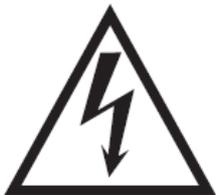
The lightning flash with symbol within the triangle is intended to warn you of a non-insulated dangerous voltage in the product's enclosure that could be of sufficient magnitude to generate a risk of electric shock to persons.
